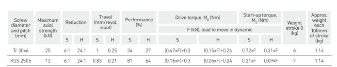
... Power required:  $P_{D}$  (kW) = 0.157x  $M_{D}$  (Nm).
