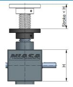
When "R" configuration gea box, if stroke is shorter that the nut length, contact us for a special design of its lubrication system, in order to ensure a right lubrication
